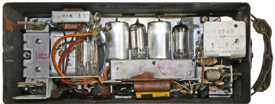
Internal view of the RCA Victor Model BP-10 with back cover removed. The 1.5V LT 'A' battery was carried on the left hand side and the 67.5V HT 'B' battery in the centre of the chassis.
