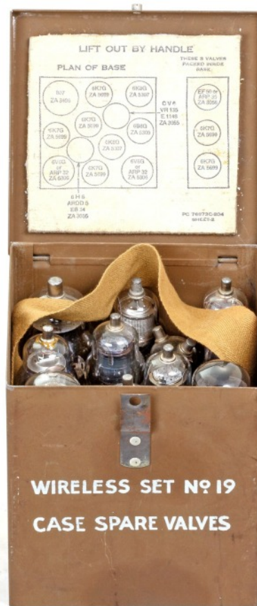
Plan of base Canadian spare valves case. Several variations have been spotted.
