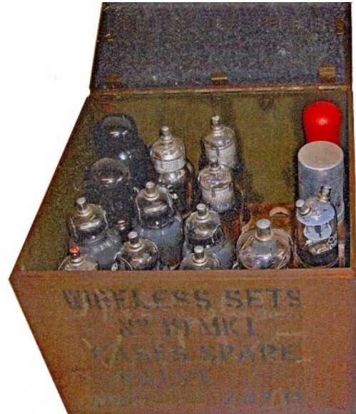
General view of WS No. 19 Mk.I spare valves case with all valves in position.
