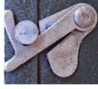
Version 1B, locking swivel catch fastened by a rivet.
