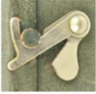
Version 1B, locking swivel catch, fastened by a rivet
