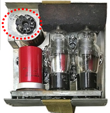
Picture of another metal spare valves base with SC inspector stamp and different valves holder retaining catches.
