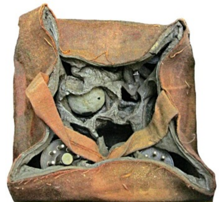
Deterioration of the sponge rubber container often transformed it into a massive block of an almost petrified substance.
