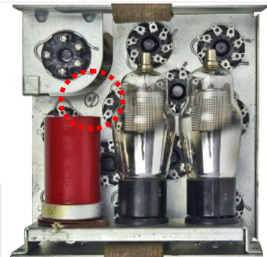
Bottom view of USA manufactured metal spare valves base. Note SC inspector stamp and valves holder retaining catches.
