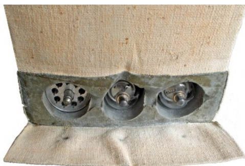
Side view of Canadian sponge rubber spare valves container. It differed with the British sponge rubber container that it had a canvas flap.
