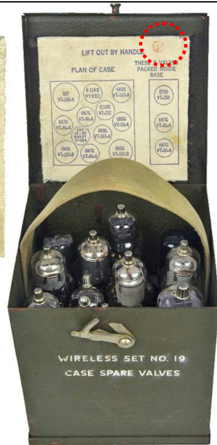
Plan of case USA produced spare valves case early version with two VT-232 valves.
