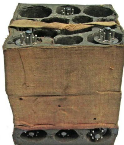
Side view of sponge rubber spare valves container showing the 3 valves packed inside.
