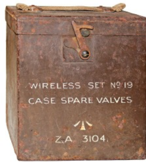
'Wireless Sets No. 19 Mk.I Cases Spare Valve' (Type 1, left) compared to later issued No. 19 Set spare valves cases 'Wireless Set No. 19 Case Spare Valves, ZA 3104' (Type 2A centre) and 'Case Spare Valve No. 4G Mk.1/1' (Type 2E right).
