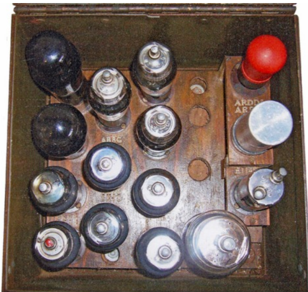
Internal view of 'Wireless Sets No. 19 Mk.I Cases Spare Valve'. The wooden base with valve holders was permanently fitted to the bottom of the steel case.
