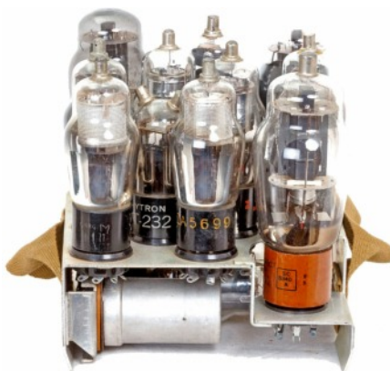
Side view of Canadian metal base with valves.
