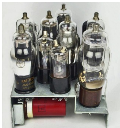
Side view of USA manufactured metal base with spare valves. This was an early production variation with two VT-232 valves.
