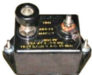
Condenser X5, 5kV was a multi purpose item used in vehicles to guard against accidental contact with overhead power lines.
