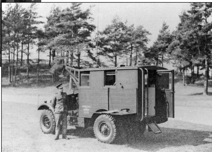
Photo right hand side: Truck, 15-cwt 4-wheeled wireless No. 1 Mk.I. This photo was probably taken later, still fitted with the existing Aerial Base No. 3 on the roof,
