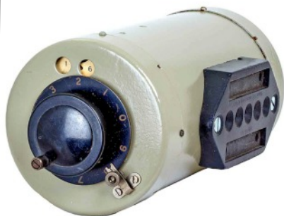
Inductance, Aerial Tuning No. 1, developed for and normally used with Wireless Set No. 19 high power.
